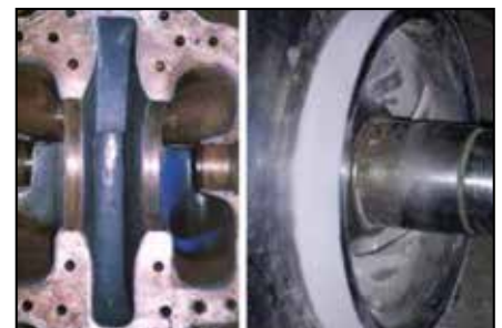
Coated sections of pump.
