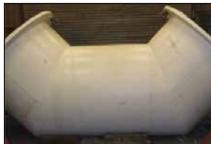
Exhaust elbow in shop laydown.
