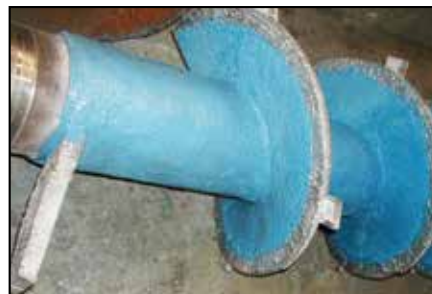
ARC MX1 applied and tips welded.
